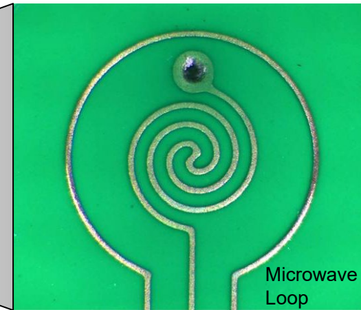
PCB Signal layer, Line width 0.1 mm
