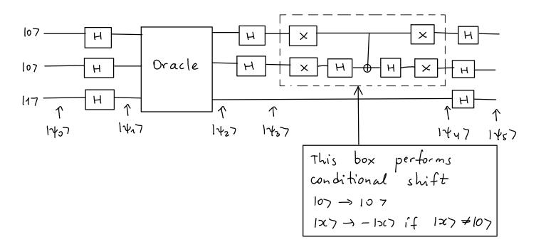
**Exercise for the class:** demonstrate that the measurement on first two qubits after this circuit will give  $|01\rangle$  when the corresponding oracle  $(x_0=1)$  is used.
