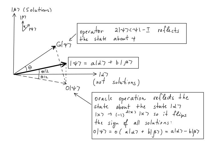
Product of two reflections is a rotation. Therefore, repeated applications of Grover iteration move vector  $\downarrow_{\psi7}$  closer to  $\mid_{\beta7}$ . The measurement will give a solution with high probability since  $\downarrow_{\beta7}$  includes all solutions.
