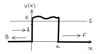
To the left of the barrier:  $\psi(x) = Ae^{ikx} + Be^{-ikx} = \sqrt{2mE}/\hbar$ To the right of the barrier:  $\psi(x) = Fe^{ikx}$ Transmission probability:  $\hat{\Gamma} = \frac{|F|^2}{|A|^2}$ Tunneling (nonclassical) region:  $(o \le x \le a)$ WKB approximation gives  $\psi(x) = \frac{C}{\sqrt{|p(x)|}} e^{\frac{1}{\pi} \int_{a}^{b} |p(x')| dx'} + \frac{D}{\sqrt{|p(x)|}} e^{-\frac{1}{\pi} \int_{a}^{b} |p(x')| dx'}$
