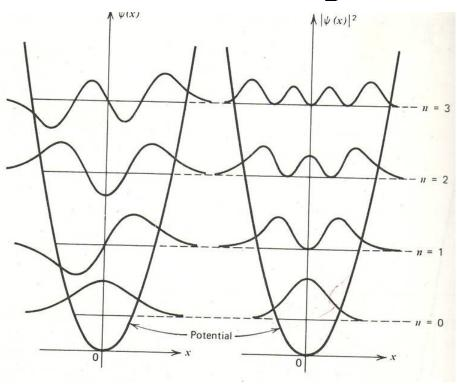
Note that the probability of finding the particle outside of classically allowed region is not zero. All wave functions extend beyond the potential energy curve representing the classically allowed maximum displacement of the oscillator.
