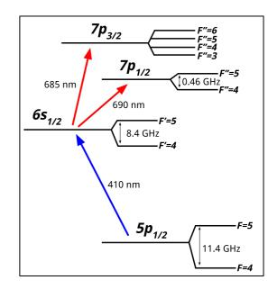
FIG. 1. Level structure of <sup>115</sup>In states relevant to the present measurements. Our two-step spectroscopic scheme requires that we overlap 410- and 690-nm (685-nm) lasers through an atom source to drive the "first-step"  $5p_{1/2}$ - $6s_{1/2}$  transition and the "second-step"  $6s_{1/2}$ - $7p_{1/2(3/2)}$  transition.
