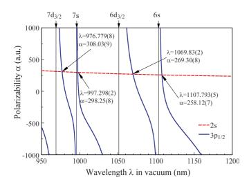
FIG. 3. (Color online) The frequency-dependent polarizabilities of the Li 2*s* and  $3p_{1/2}$  states. The magic wavelengths are marked with arrows. The positions of the resonances are indicated by vertical lines with small arrows on top of the graph.
