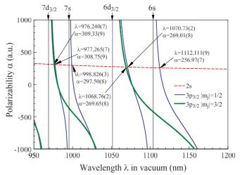
FIG. 4. (Color online) The frequency-dependent polarizabilities of the Li 2s and  $3p_{3/2}$  states. The magic wavelengths are marked with arrows. The positions of the resonances are indicated by vertical lines with small arrows on top of the graph.
