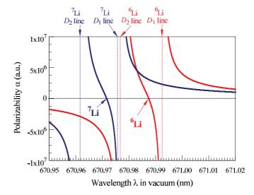
FIG. 5. (Color online) The frequency-dependent polarizabilities of the ground state of <sup>6</sup>Li and <sup>7</sup>Li. The tune-out wavelengths are marked with arrows.
