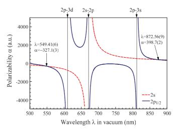
FIG. 1. (Color online) The frequency-dependent polarizabilities of the Li 2s and  $2p_{1/2}$  states. The magic wavelengths are marked with arrows. The positions of the resonances are indicated by vertical lines with small arrows on top of the graph.
