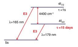
FIG. 1. (Color online) Energy levels and radiative lifetimes of low-lying levels of Ag-like Nd<sup>13+</sup>.
