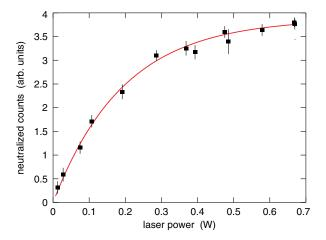
FIG. 3. Neutral atoms detected as a function of transverse laser beam power. The solid red line is a fit with the analytical rate equation solution  $N(W_0)$ , as described in the text.
