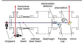
FIG. 1. Sketch of the combined collinear and transverse laser spectroscopy setup (top view) with an overlap region of 730 mm. The ion beam is indicated by a blue line, the laser beams by red lines.
