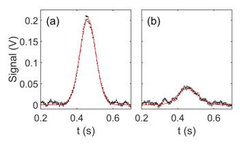
FIG. 3. Absorption spectra for (a) parallel polarization and (b) perpendicular polarization, at a detuning of  $\Delta/2\pi=107.5~{\rm cm}^{-1}$ . The black dots are experimental data while the red curve is the least-squares Gaussian fit to the data. With a laser frequency scan rate of  $\sim 2.0~{\rm GHz/s}$ , the total frequency width of these plots is  $\sim 1.0~{\rm GHz}$ . The ratio of peak heights at this detuning is  $S_{\parallel}/S_{\perp} \sim 5.35$ .
