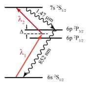
FIG. 1. Energy level diagram of atomic cesium, showing the states relevant to this measurement. Atoms are excited from the  $6s^2S_{1/2}$  ground state to the  $7s^2S_{1/2}$  excited state by two-color, two-photon excitation. We collect fluorescence photons at 852 nm from the second step of the spontaneous decay of atoms from the 7s state to the ground state by way of the  $6p^2P_{3/2}$  state.
