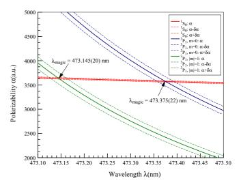
FIG. 1. Calculated polarizabilities for  $5s^{2-1}S_0$  and  $5s5p^{-3}P_1$ , m = 0, and |m| = 1 levels and corresponding magic wavelengths.
