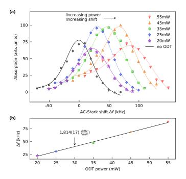
FIG. 3. (a) Sample absorption spectroscopy scans for varying powers of an ODT at a wavelength of 473.65 nm for the  $\pi$  transition. The AC Stark shift axis is centered with respect to a reference scan without ODT (black solid line). Each scan is fitted to a Voigt plus linear model (see the Appendix). (b) AC Stark shift vs ODT power. At this wavelength, the Voigt centers increase in frequency with the ODT beam power and result in a positive differential Stark shift coefficient (DSSC).
